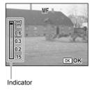
After the focus is corrected, press the OK button to set the focus position and return to the normal capture screen.
